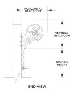
Universal mount 3" deep 12 gauge galvanized steel guides require no pre-installation modifications for wood, steel, concrete or filled masonry block applications.
